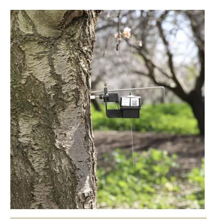
Dendrometers used for tracking changes in stem water potential in real time
