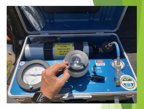
Pressure bomb method for tracking water stress
